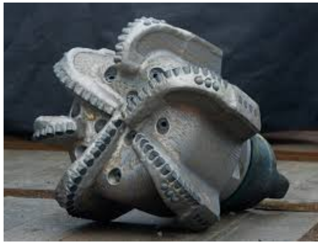
Figure 2. A drill bit that crushes the rock with teeth of tungsten carbide and synthetic diamond. Fracking lubricant mud is pumped down the pipes and exits jets on the bit. The mud and crushed rock are forced to the surface in the outer annular region between the drill bit and casing.
