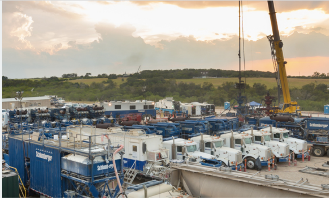
Figure 3. A drilling rig site. A typical well site requires about 1,500-3,000 round trips by heavy trucks to support the water, sand, and other chemicals. The drilling goes on 24/7. A typical complete drilling and fracking operation can take 1-2 months. A well site footprint needs about 5 acres. (Schlumberger).
