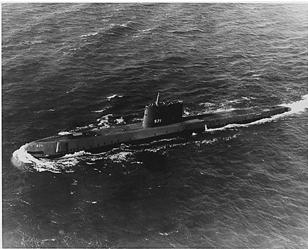
Figure 1. The Nautilus submarine. The 10 MW nuclear reactor design was an LWR; a design that dominates world reactor designs today. The Nautilus was launched in 1954 and set records for speed (25 knots), underwater submersion (2 months), and diving under the Arctic Ice Cap [14].
