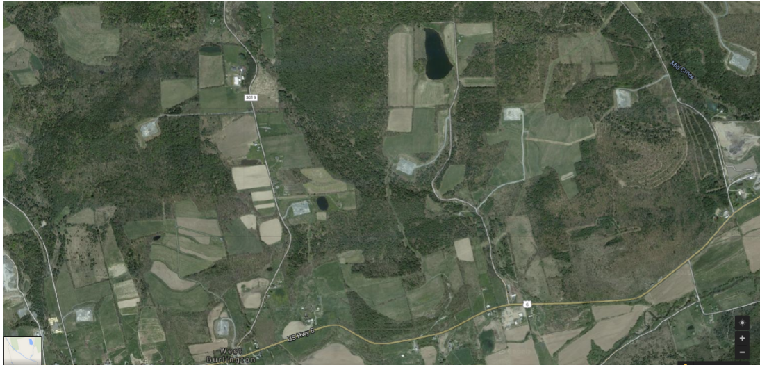
Figure 3. This roughly one square mile of Bradford County Pennsylvania land shows eight completed well pads (small gray squares) and two retention ponds not yet cleared. Notice the narrow winding country roads and proximity to farmhouses. ( www.Google Maps.com )
