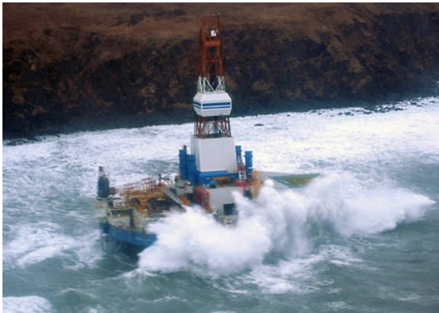
Figure 5. The exploratory oil drill rig Kulluk beached in Aleutian Islands by severe winter weather. The rig is 250 feet high, has a drill depth of 20,000 feet, and is not capable of motoring in the sea.
