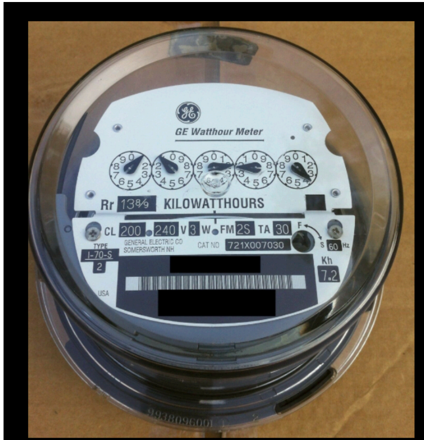
Figure 5. Residential power meter by GE Corp.
