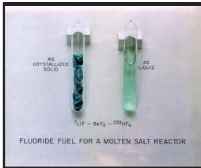
Figure 4. Molten salt and fuel: \text{LiF} - \text{BeF}_2 - {}^{233}\text{UF}_4
