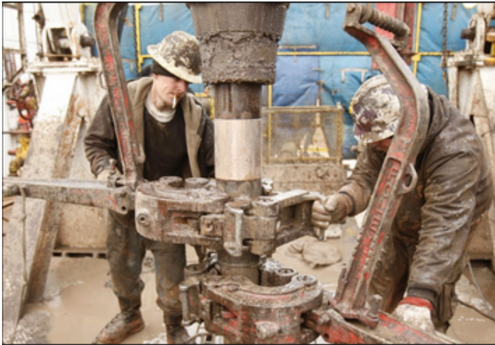
Figure 2. Rig workers in slippery conditions use large wenchers to couple 50 foot threaded pipe sections. (www.cnn.com)
