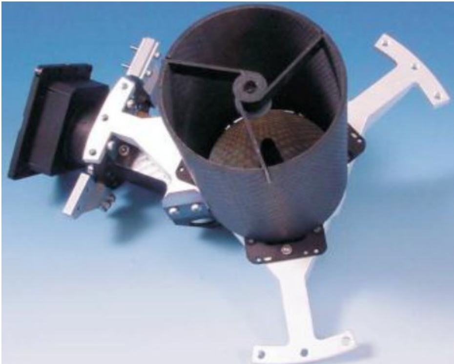
Telescope made of material, which has a very low thermal expansion.
