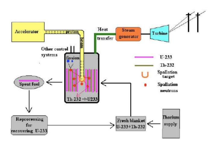
Schamtic of an Accelerator Driven Sub-critical System to produce electricity as well as breed fissile Uranium-233
