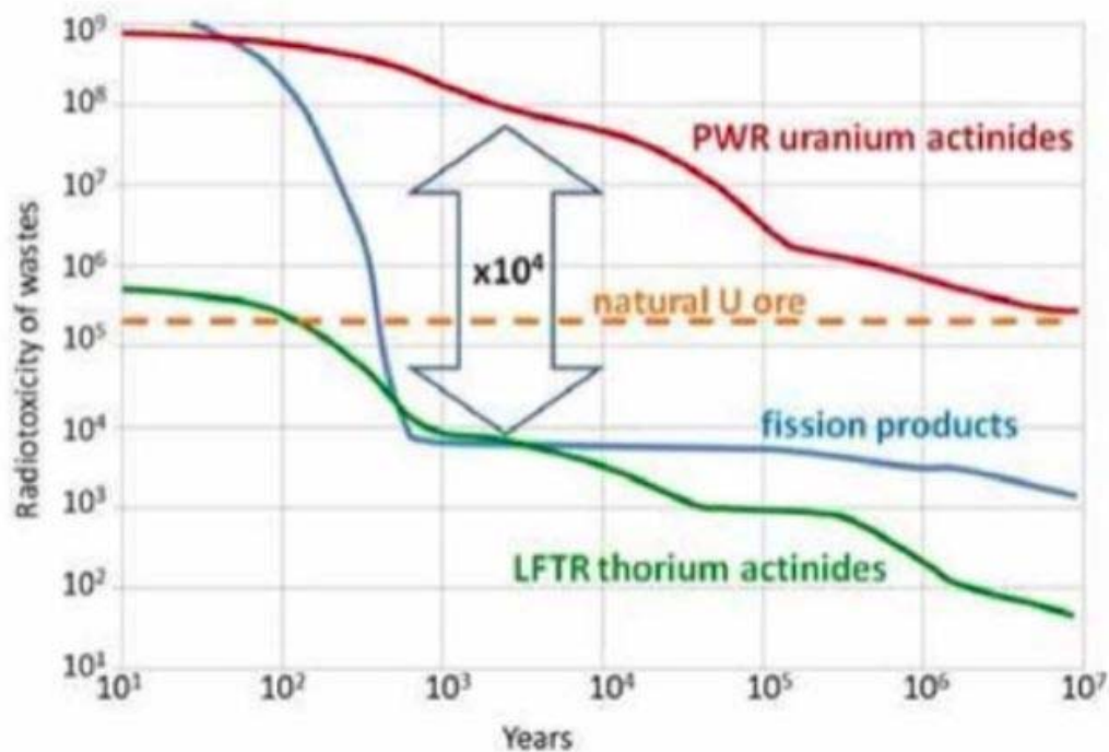
Radiotoxicity of LFTR (thorium MSR) and PWR wastes over time
