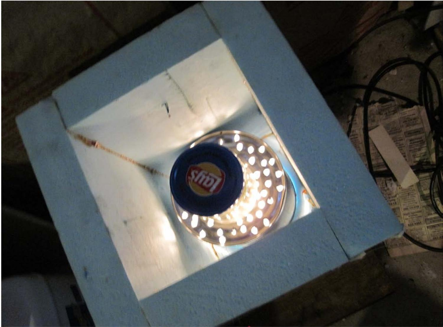
**PCT oven: a light bulb-heated, “blue board” box, with diode T sensor/op amp/SCR temp controller**
