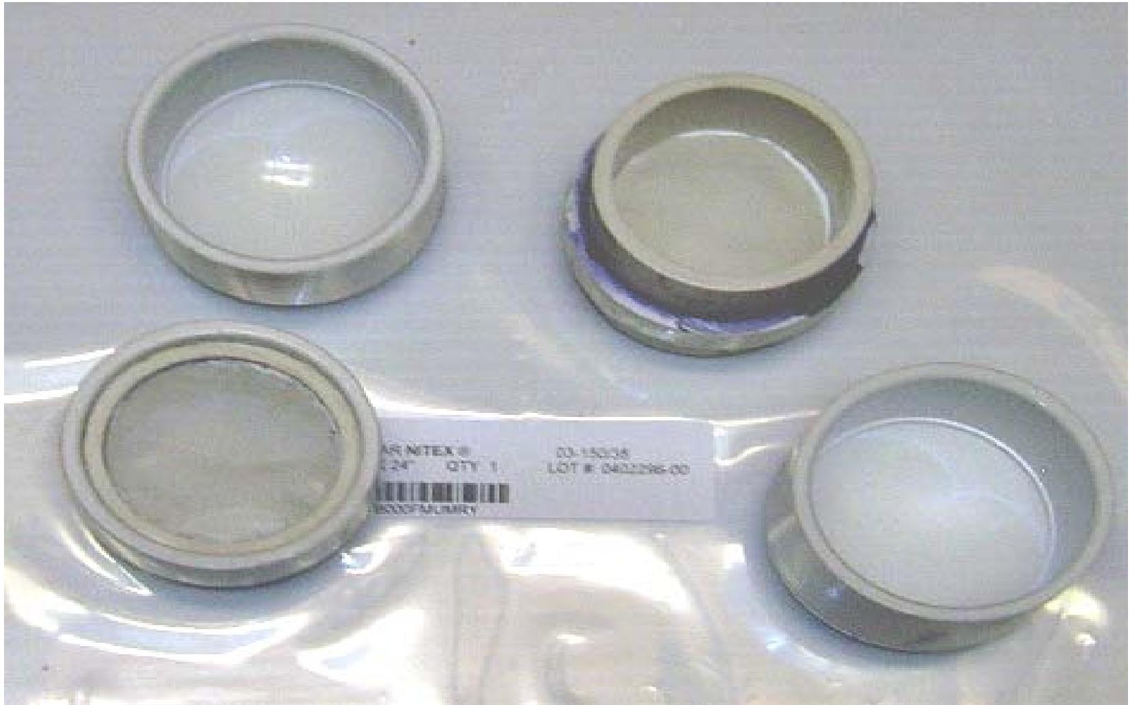
PCT sample screens: 150 & 75  $\mu$  NITEX™, silicone glue, & 2" PVC pipe fittings
