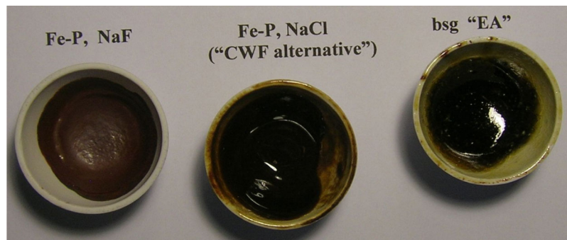
Fig. 3. Direct vit products (everything is mixed together and melted in the crucible) Fe-P — sodium fluoride plus H_3PO_4/Fe_2O_3 (a glass composite material); CWF alternative 4 = equivalent amount of NaCl plus H_3PO_4/Fe_2O_3 (a genuine glass); bsg EA = remelt of DOE's benchmark borosilicate glass.
