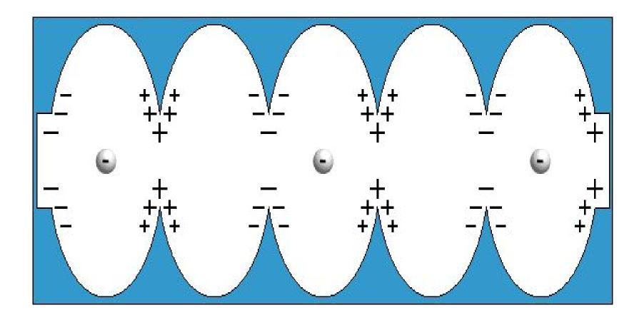
For continuous wave operation the resonant cavity material needs to be made out of superconducting niobium since the surface resistance is a million times smaller there by reducing the wall losses (please refer to my earlier TEA conference presentations)
