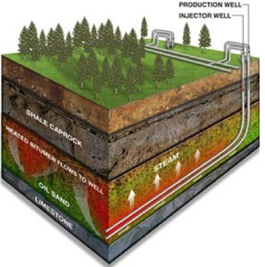
~3 barrels of steam per barrel of bitumen
