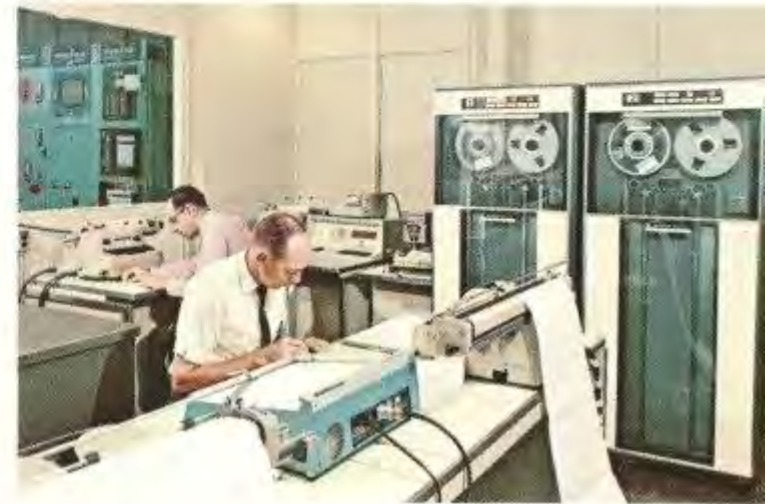
Information which is needed immediately by the reactor operator is displayed on the main control panel (above). Auxiliary instruments not requiring constant surveillance are located in other areas. Below, a digital computer and data handling equipment are utilized to provide current information on important variables within the reactor system.
