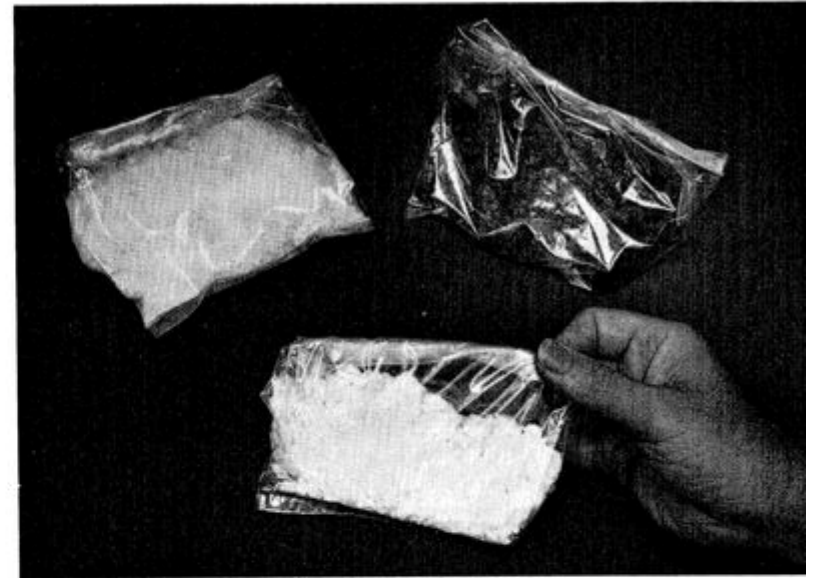
Fluoride salts used in the MSRE are displayed (above) in a solid state. From the left are the coolant (lithium-beryllium fluoride), fuel solvent (lithium-beryllium-zirconium fluoride) and fuel concentrate (lithium-uranium fluoride). Below, a horizontal kiln is used in the densification of lithium fluoride.
