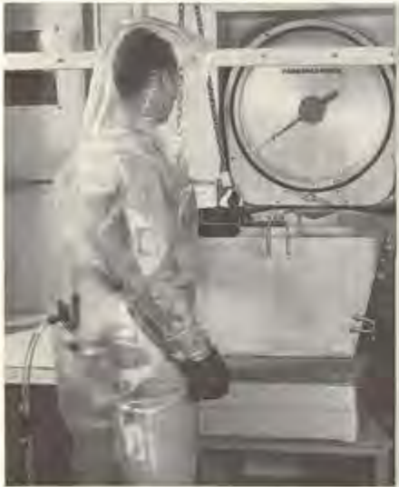
Protective clothing is required in the raw materials handling area of the Fluoride Production Facility (above) to avoid inhalation of the toxic salts. Below, a diagram of the fuel processing system. At right below is the fuel processing containment cell located in the reactor building.
