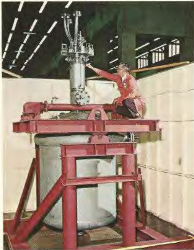
The completed reactor vessel above is shown during inspection and before being installed in its containment cell. On page 3, a simplified flow diagram of the reactor's principal components.
