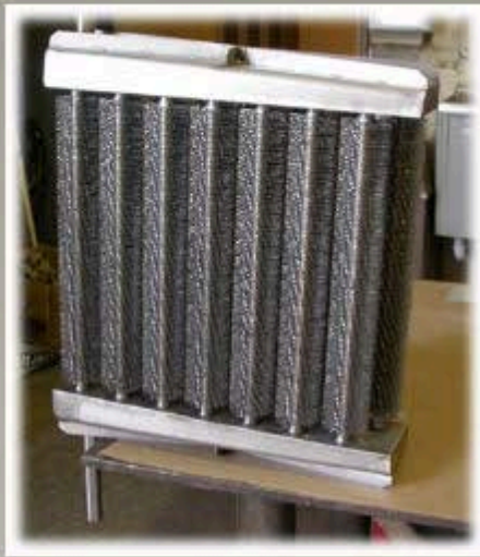
Finned tube air cooler - 200 kw
