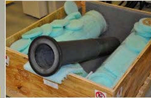
SiC test section - 600 graphite spheres 1.25 kw/sphere (max)
