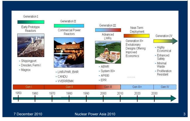
Gen II (most existing units, these work well); Gen III/III+ (moving to FOAK, size increase); Gen IV (R&D/SMA)
